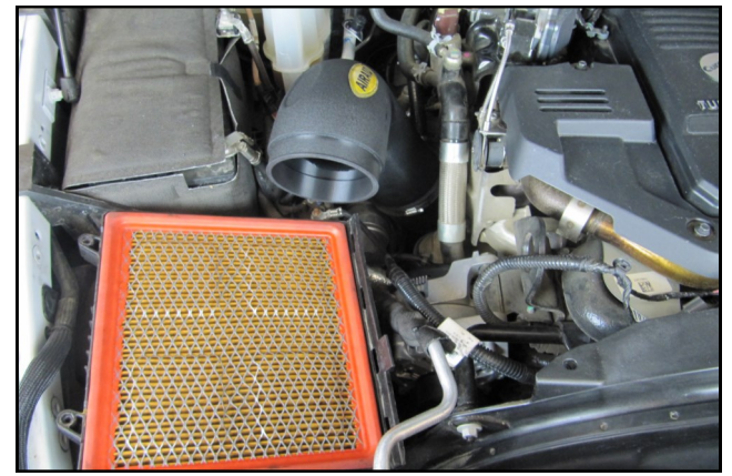
5. Slide the Airaid intake tube into the turbo inlet but leave the clamp loose for now.
