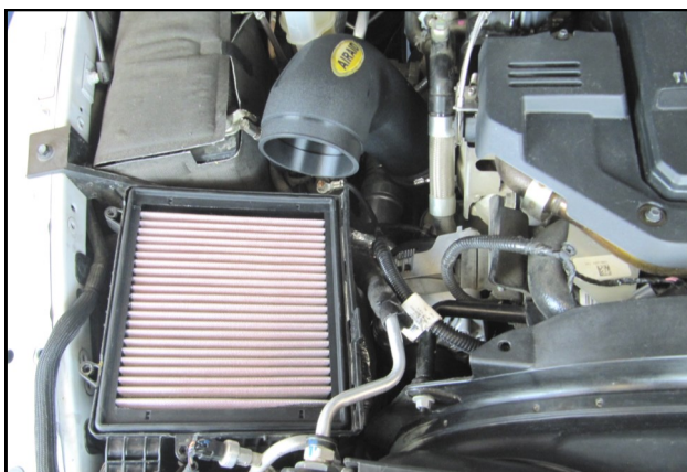
6. If you are installing an Airaid Jr. kit, install the Airaid Premium Filter at this time.
